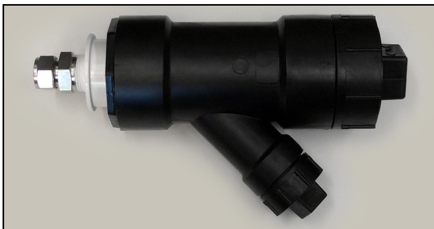
Figure C-6. Zero Flow calibration chamber — assembled
